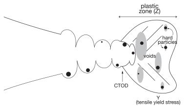
The crack must open to a certain extent to accommodate the damage at the crack tip so that the crack can advance.
