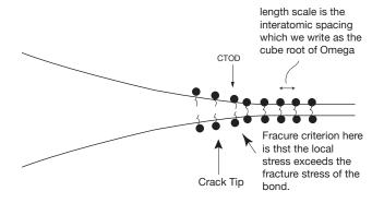
(ii) The crack tip opening displacement (CTOD)
